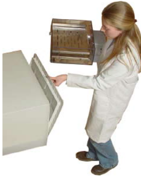
TRANSPORT CHAMBERS are designed for moving cultures without disturbing conditions inside. They are light enough to carry and balance on one hand.
